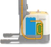
**Crown Regen Lower System** (available on SP 4000) captures lost energy and returns it to the battery. This equates to fewer battery changes, longer shifts and reduced costs.
